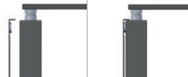
mounting by magnets and small hooks
