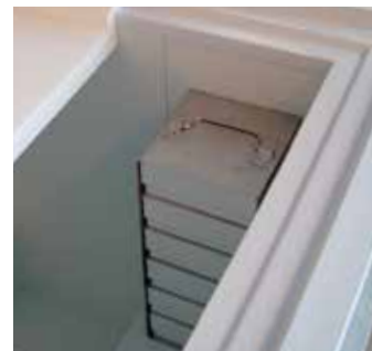
Inner lids (left hand side) which are mandatory for optimized function
